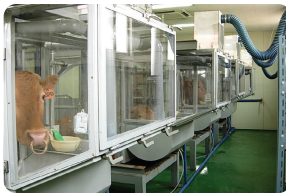
Measurement of methane gas emission of Hanwoo using respiration-metabolism chambers
